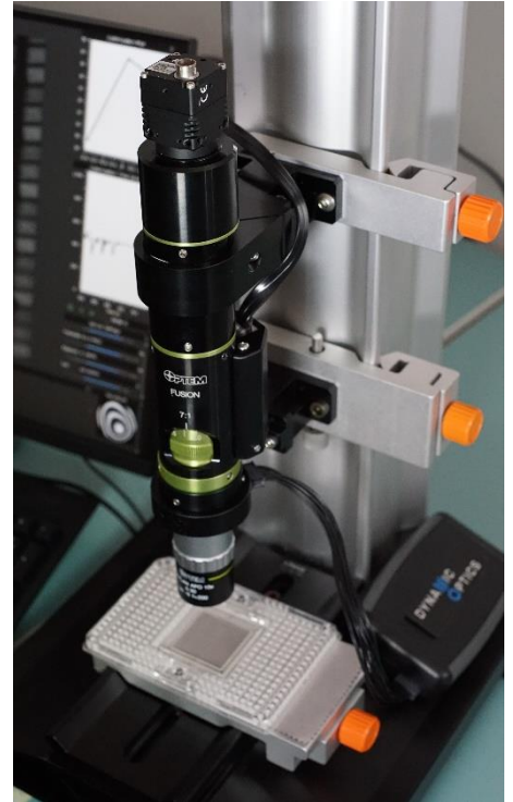
Fig. 4: Image of a brightfield microscope objective with deformable lens.
