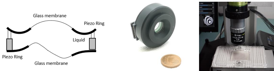
Fig. 3: left) cross section of the deformable lens. Center) image of the deformable lens (10mm clear aperture). Right) Deformable lens mounted on a microscope objective.
